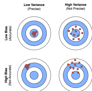
Figure 10.4: Graphical representation of the quality of an estimator: predicted values represented on a target centered on the value to be estimated for different bias/variance situations. Credit(Picture): Sebastian Raschka
